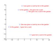
The figure shows a 2-dimensional PCA projection of the LSTM hidden states that are obtained after processing the phrases in the figures. The phrases are clustered by meaning, which in these examples is primarily a function of word order, which would be difficult to capture with a bag-of-words model. The figure clearly shows that the representations are sensitive to the order of words, while being fairly insensitive to the replacement of an active voice with a passive voice.
