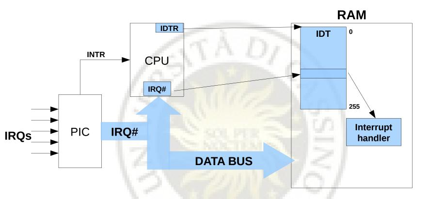
In practice the CPU automatically jumps to (execute) the handler of the device which generated the interrupt
