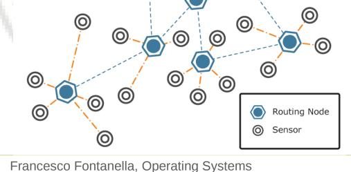
A WS is a very little computer: CPU, RAM, ROM, I/O (sensors, wireless communications)
