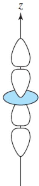
Sigma bonding interaction between two ligand orbitals and metal d_{z^2} orbital
