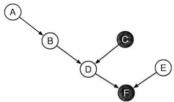
Inference in a polytree scales linearly in the number of nodes and the sizes of their conditional probability tables (CPTs). For the belief network shown above, consider how to efficiently compute the posterior probability P(E|C,F). This can be done in four consecutive steps in which the later steps rely on the results from earlier ones.
