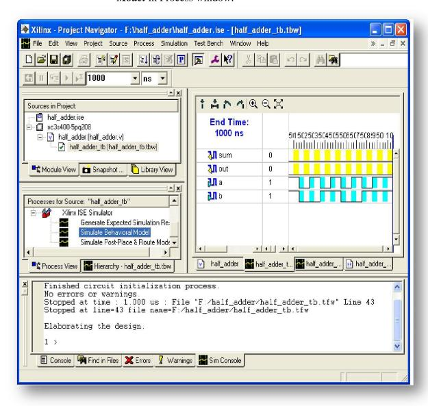
Verify the design in wave window by seeing behavior of output signal with respect to input signal.
