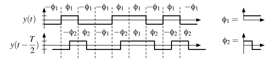
Without a delay, the signal decodes to channel 1.
