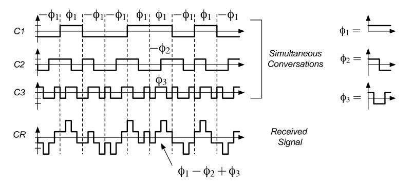
The received signal at one interval contains these superimposed codes from each channel, weighted by channel gain, transmit power, etc
