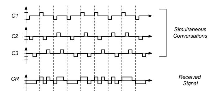
Here there are four time slots. C1 only transmits during the first time slot, C2 the second time slot, etc.
