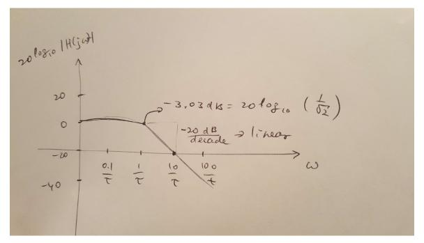
If  $20\log|H(j\omega)|>0 \rightarrow$  The signal is amplified If  $20\log|H(j\omega)|<0 \rightarrow$  The signal is attenuated
