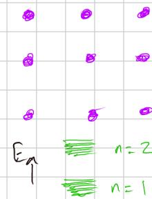
N atoms brought together causes E-levels to split N times
