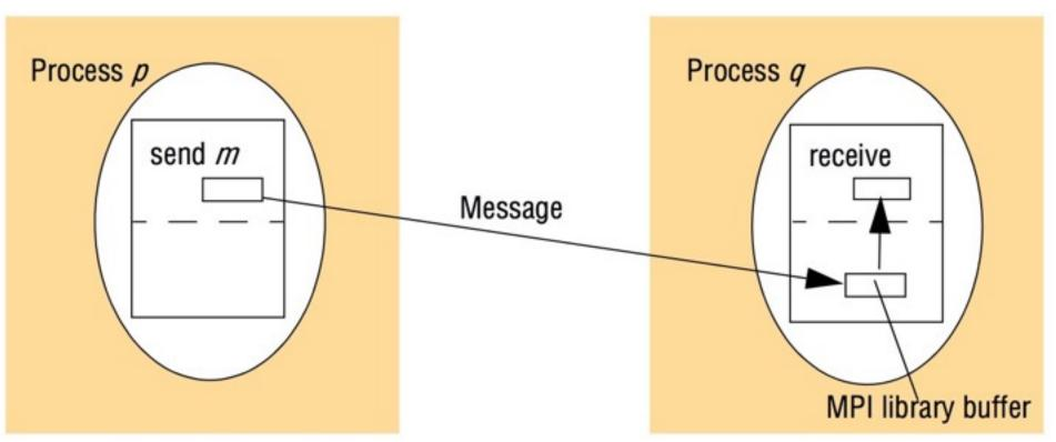
• An MPI library buffer in both the sender and the receiver is used to hold data in transit
