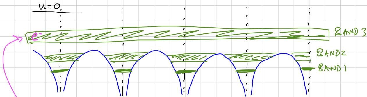
Generally, an  $e^-$  will be in an "upper" or higher energy band and thus is effectively like a particle-in-a-box with:
