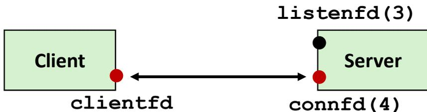
*3. Server returns `connfd` from `accept`. Client returns from `connect`. Connection is now established between `clientfd` and `connfd`*
