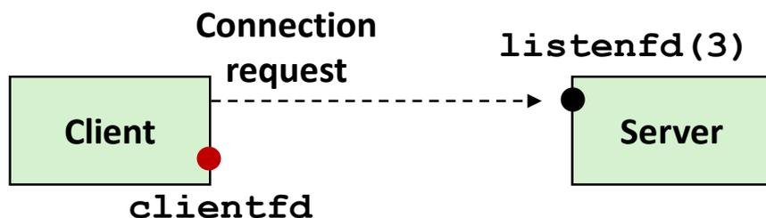
*2. Client makes connection request by calling and blocking in `connect`*
