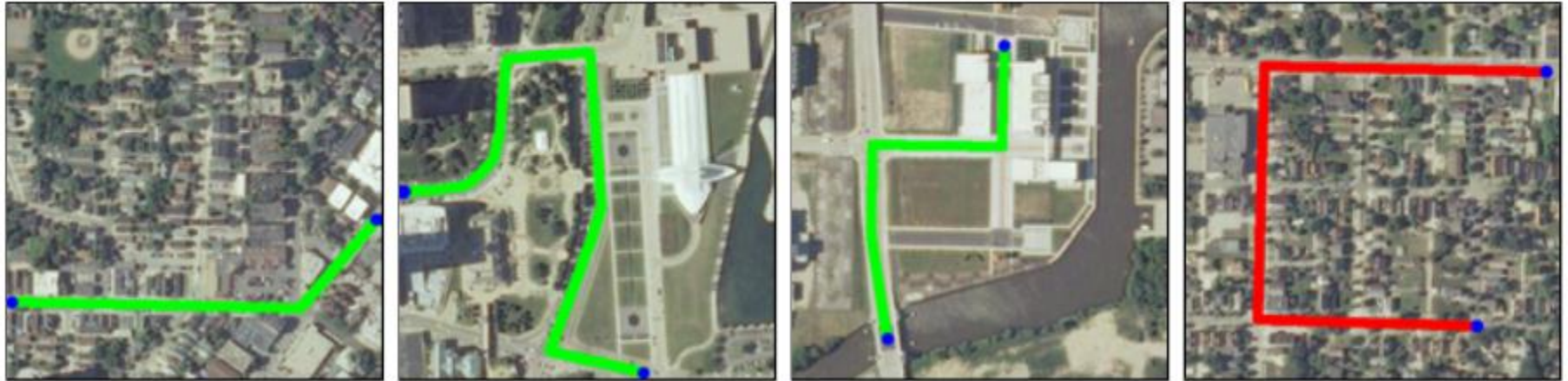
Fig. 6.4 Illustration of Learning to Plan . Given a set of training paths (green) between given start and end locations, the task consists of learning a prediction function that find similar paths in new images (red), e.g., preferring larger roads over smaller ones and avoiding water and vegetation. (Image Source: WisconsinView.org, SSEC).
