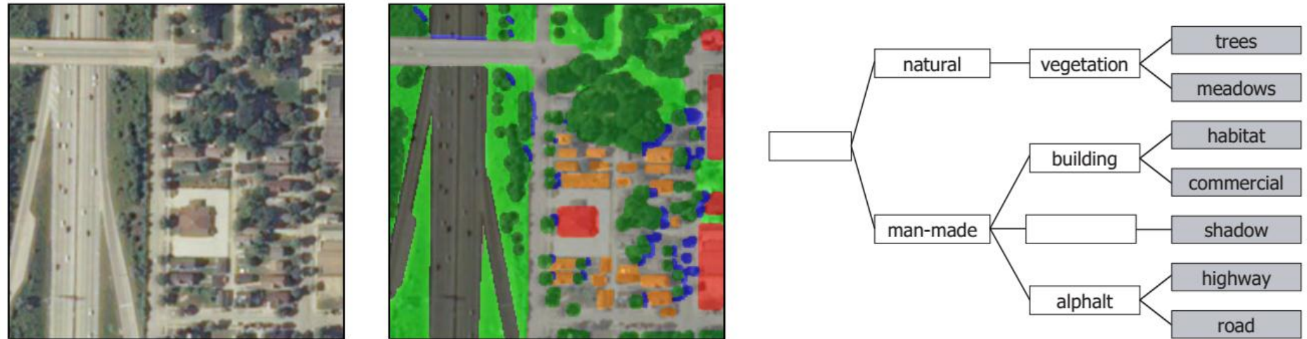
Fig. 6.6 Illustration of automatic remote imaging ground survey [153]. Each pixel of a multispectral aerial image (left) is classified into one class of a seven class hierarchy (right). Outputs (middle) are color coded: trees (dark green), meadows (light green), highway (dark gray), road (light gray), residential (orange), commercial (red), and shadow (blue). (Image Source: WisconsinView.org, SSEC).
