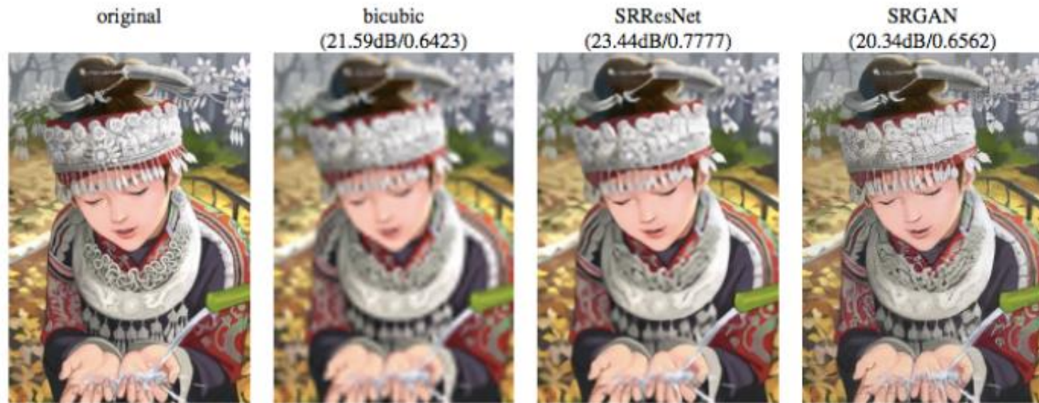
Figure 4: Ledig et al. (2016) demonstrate excellent single-image superresolution results that show the benefit of using a generative model trained to generate realistic samples from a multimodal distribution. The leftmost image is an original high-resolution image. It is then downsampled to make a low-resolution image, and different methods are used to attempt to recover the high-resolution image. The bicubic method is simply an interpolation method that does not use the statistics of the training set at all. SRResNet is a neural network trained with mean squared error. SRGAN is a GAN-based neural network that improves over SRGAN because it is able to understand that there are multiple correct answers, rather than averaging over many answers to impose a single best output.
