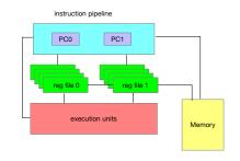
The OS may handle a large number of concurrent SW threads, but only one per HW thread can run simultaneously. one at a time
