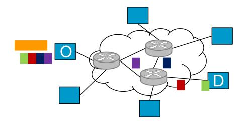
Real networks constrain throughput between end systems, introduce delay and can even loose packets
