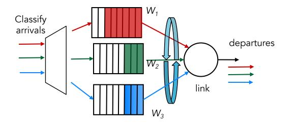
class *i* will get a fraction of service equal to  $w_i / \Sigma w_j$  where the sum is over all classes with packets queued for transmission
