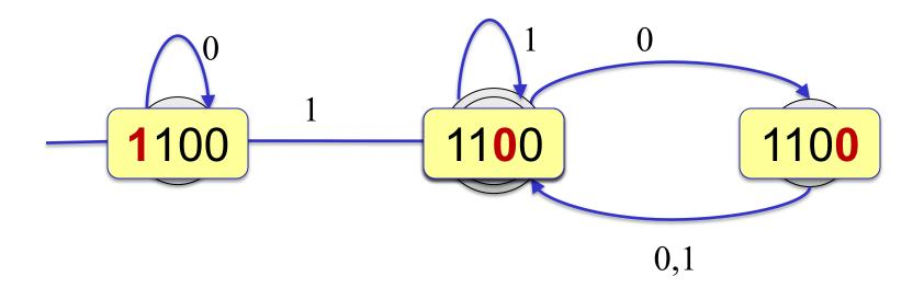
The machine accepts a string if the process ends in a double circled state
