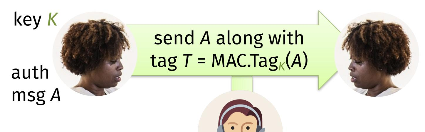
MACs stop an actively malicious Mallory from: - injecting a new message and tag (A\*, T\*) - tampering with an existing one
