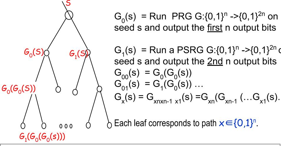
$f_{s}(x) = G_{x}(s) = LSB(label of leaf x) e.g. f_{i}(0000) = LSB(G_{0}(G_{0}(G_{0}((s)))))$   $(G_{0}(G_{0}((s)))))$ Set PSRF family F= {F<sub>n</sub>} and F\_{n}={f\_{s}}\_{|s|=n}
