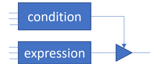
Tri-state buffer inferred based on 1'bz assignment
