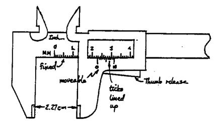
In the figure above, the measured object has a total thickness of 2.27 cm.
